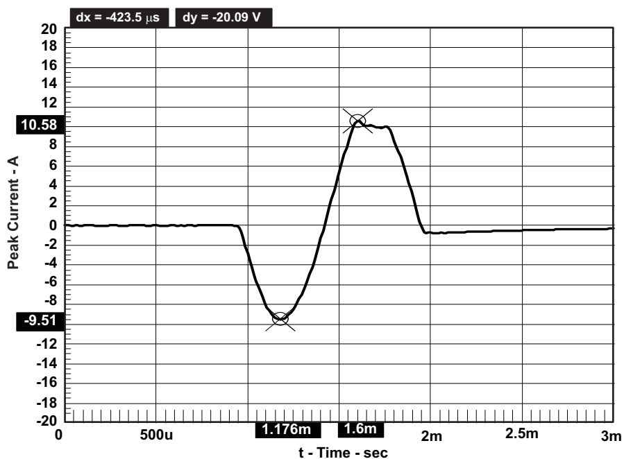
Figure 19. High-Current Protection (SE)
